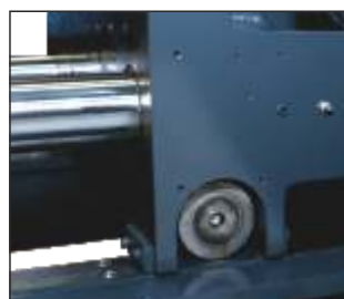
Moving platen supported on anti-friction roller bearings
